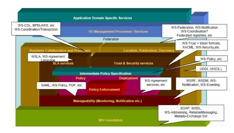
Figure: A component architecture to support the TrustCoM framework for security, trust and contract management of dynamic VO.
