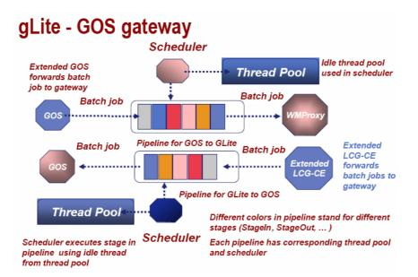
Figure: The gateway developed in the EUChinaGrid project between the gLite middleware used in the European EGEE project and the GOS middleware used in CNGrid in China.
